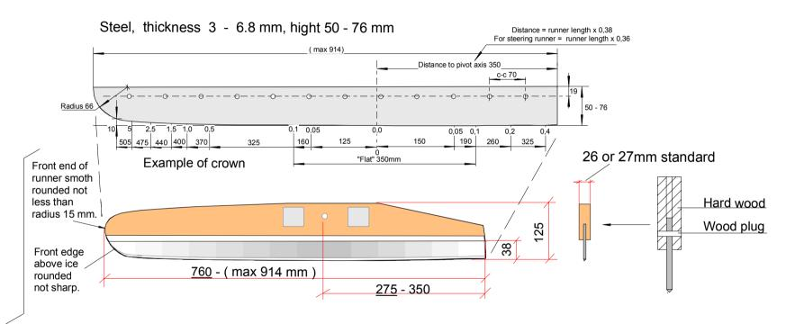
Both of this specs. are designed to prevent, sharp leading edges on runners, witch might cut a sailor in a collision.
